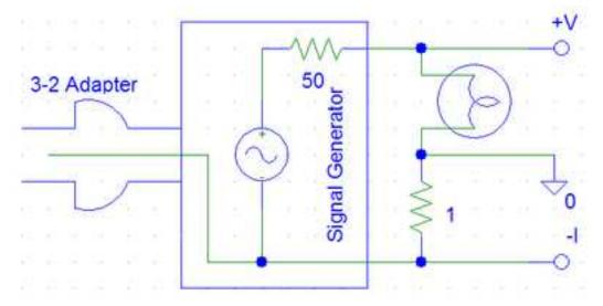
Note the use of the 3-2 prong adapter to float the signal generator (allow it to have a different ground voltage than the oscilloscope). The ground shown in the diagram (labeled 0) should be shared with the oscilloscope.
