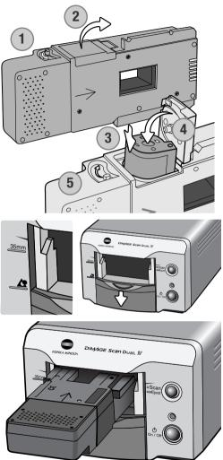
When using the APS adapter, if the scanner makes a strange sound or the film-advance warning appears, eject the APS adapter immediately (p. 21) and do not reinsert it. Contact a Konica Minolta service facility.
