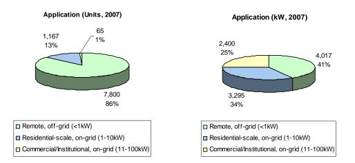
All turbines under 1kW, and 90% of turbines equal to 1kW, were assumed to be off-grid where confirmation was unavailable. Several models sold are adjustable to either on- or off-grid purposes.
