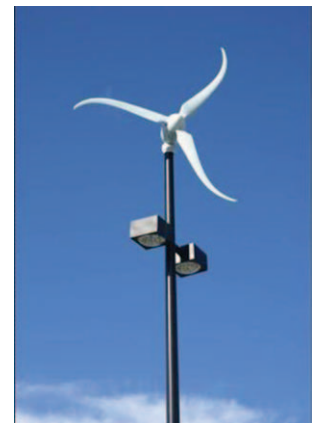
Skystream 1.8kW turbine dual-use on lamppost
