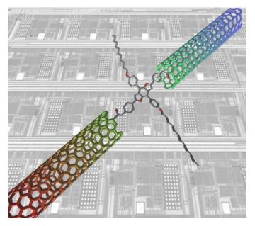
Illustration of a new method to wire molecules directly into nanometer-scale gaps in conducting single-walled carbon nanotubes. Credit: Columbia University.
