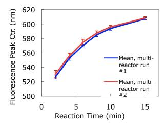
time over 160 samples, we were able to determine kinetic rate orders, activation energies, and pre-exponential factors for nanocrystal growth. These results demonstrates the power of automation to enable rapid refinement and detailed investigation of synthetic methods.
