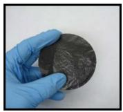
Figure 2. SWCNT paper that is used to make an anode
