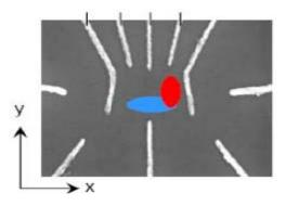
Micrograph of GaAs single-electron transistor used in the experiments. The electrodes are approximately 50 nm wide. Adjustments to the voltages on the electrodes change the potential in the way illustrated by the red and blue ovals. For the blue the potential rises more rapidly along the y direction, so the energy of the first excited state along y increase going from red to blue.
