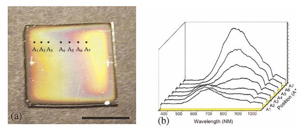
Figure. (Color) Antenna length effect. (a) Interference colors from the random array of MWCNTs. A1–A7 are the selected positions where the length and optical measurements were carried out. Scale bar, 1 cm. (b) Reflected light intensity vs radiation wavelength measured in selected points on the sample shown in (a).
