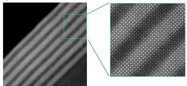
Fig. 1 Superlattice of  $(LaMnO_3)_6/(SrMnO_3)_6$  synthesized by oxide MBE at the CNM, Argonne. Image: Amish Shah, Jian-Min Zuo,
