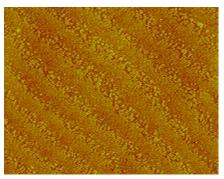
Fig. 2 AFM image of a surface of a superlattice of  $(LaMnO_3)_1/(SrMnO_3)_1$  synthesized by oxide MBE at the CNM, Argonne. Image: Tiffany Santos
