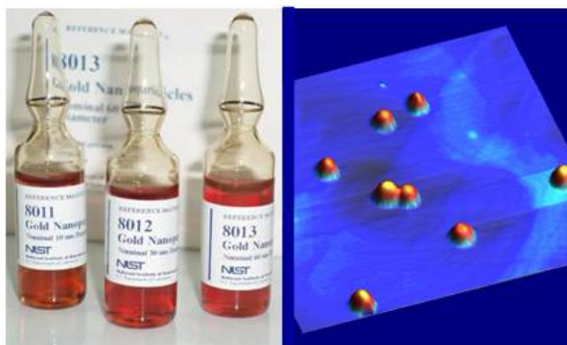
Figure 1. NIST gold RM units and an image of individual 60 nanometer gold particles.
