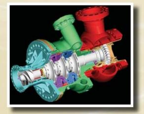
**Impact:** This alloy enables a revolutionary two stage liquid hydrogen turbopump that achieves major objectives of the Integrated High Payoff Rocket Propulsion Technology (IHPRPT) Initiative for dramatic increases in thrust-to-weight, reliability and affordability of liquid rocket engines for improved access to space. Additional applications are being pursued with industrial partners, including turbopump housings and large pipes in liquid rocket engines, aircraft wheels and automotive parts.
