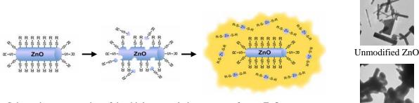
Schematic representation of the thiol encapsulation process of nano-ZnO
