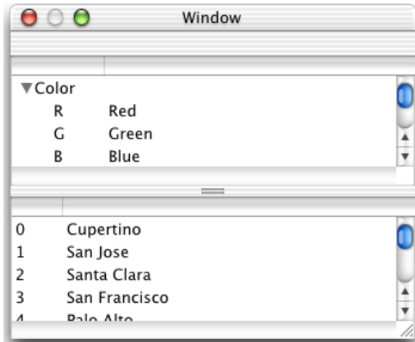
Figure 4-6 A split view that contains an outline view and a table view
