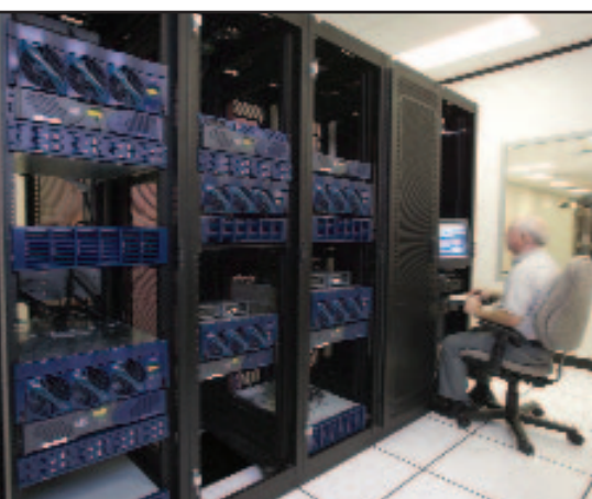
The SGI Origin 300 video server is controlled by Harris automation. Harris also controls the SGI Media Server for broadcast MPEG-2 video servers.
