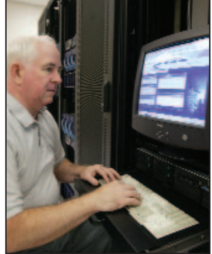
Buster Hampton works on the MassStore, which manages and accesses the broadcast data infrastructure while providing the interface for moving broadcast data between the various storage systems.
