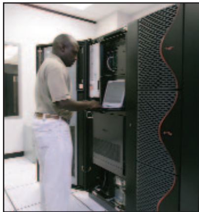
Horace Eberhart is shown working on GPB's main disk storage environment, the Hitachi Data Systems 9980V.
