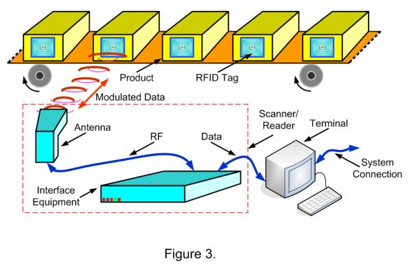
**Figure 3.**, shows a typical industrial RFID application where a conveyor belt of products is having each RFID tag scanned to detect the previously written product identifier, for example: -
