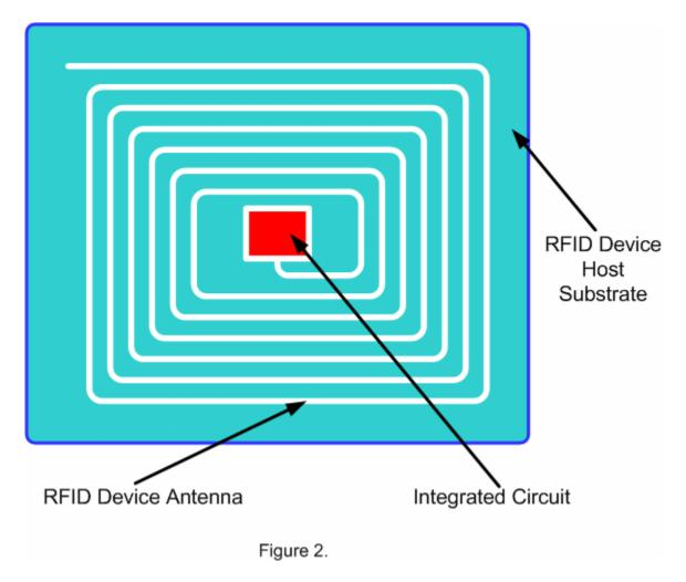
The typical RFID tag portrayed in **Figure 2**., comprises a host substrate which is typically, but not exclusively, a flexible plastic (polymer), with an attached flexible etched aluminium alloy, or conductive ink antenna, plus a small (few millimetres square) attached integrated circuit connected to the antenna. The whole assembly is typically 30 millimetres square, a fraction of a millimetre thick, and is encapsulated so that it forms a flexible durable, attachable label.
