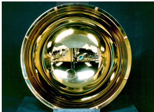
Hemi-ellipsoid reflectometer , one of the critical hardware items of the Reflectance Laboratory
