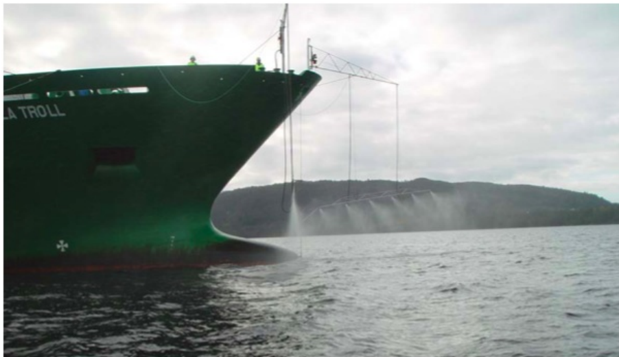
Figure 6.2: Newly developed system for application of dispersants from a vessel.
