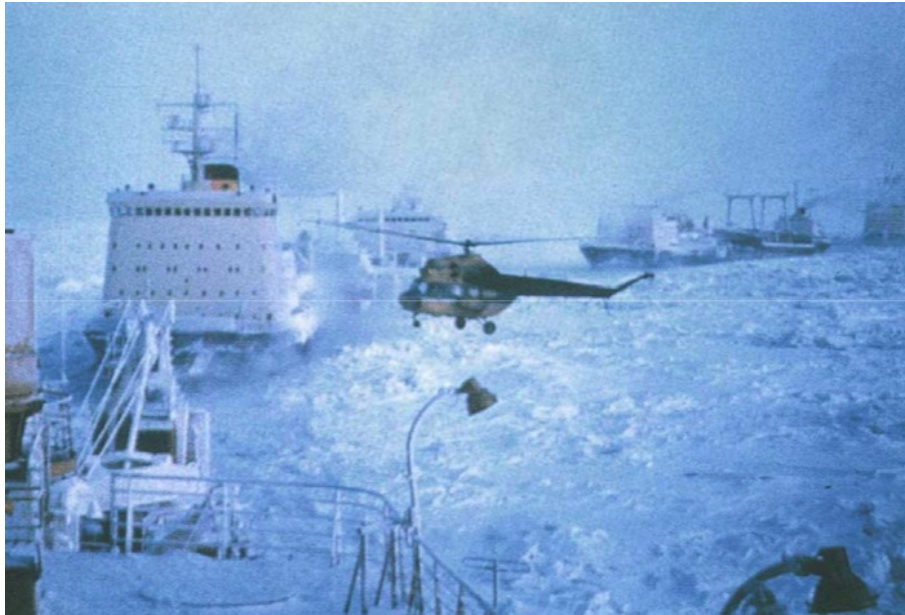
Fig. 2.7. Escorting of cargo ships under heavy ice conditions each ship being towed by a single icebreaker
