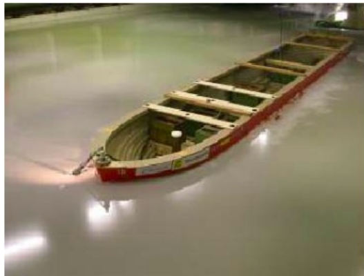
Model tests with angled ice rift
