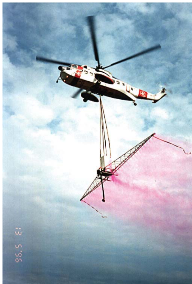
Figure 4.17 Testing of the Norwegian Response 3000 D helicopter bucket.
