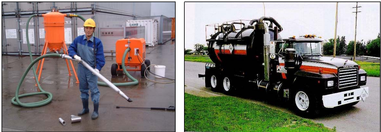
Figure 4.7 Vacuum skimmers are often confused with air conveyors. The driving force for a vacuum unit is the pressure drop in the hose transferring the product, while the driving force for an air conveyor is the drag from air on the product to be transferred.
