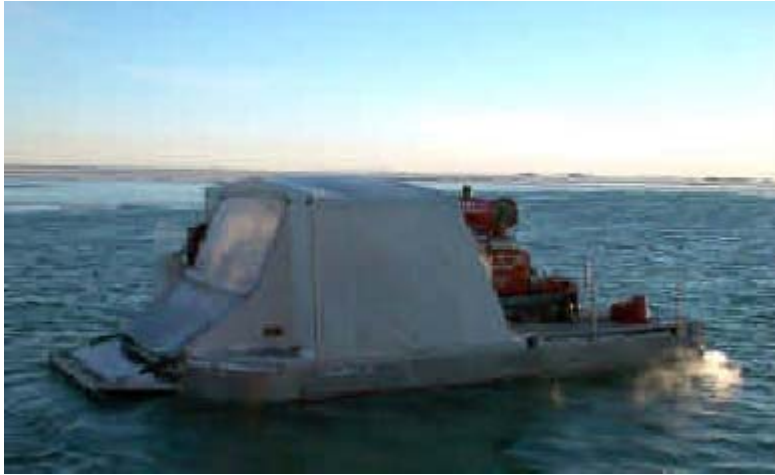
Figure 2.2 The MORICE work platform during sea trials in Prudhoe Bay, Alaska, with a heated enclosure to avoid icing and freezing of equipment (Jensen, 2004).
