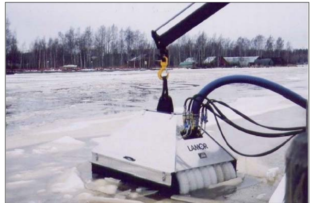
Figure 2.3 a-b a) Lamor GT 185 modified with rotating brush to improve flow over weir b) Lamor Arctic Skimmer LAS 125 W/P
