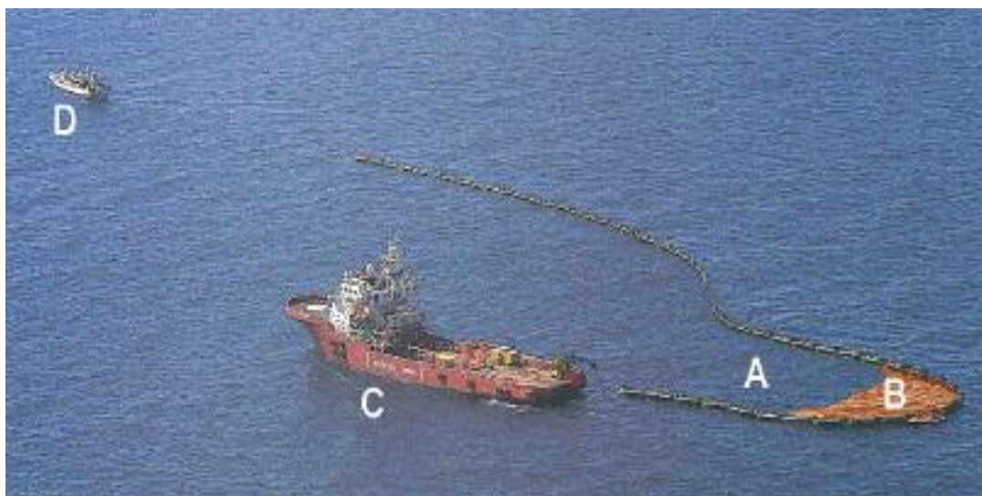
Figure 4.1 Offshore oil recovery system standardized by NOFO. A: boom; B: Transrec skimmer; C: main vessel; D: towing vessel.
