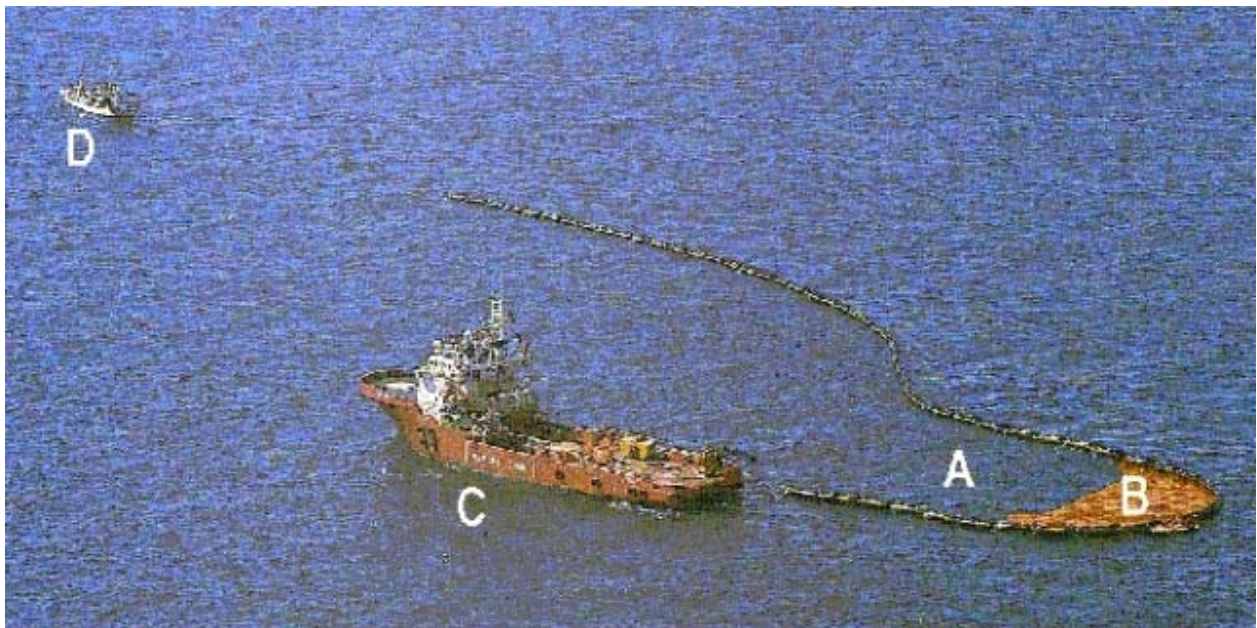
Figure 6.1 Offshore oil recovery system standardized by NOFO. A: Boom; B: Transrec skimmer; C: Main vessel; D: Towing vessel.
