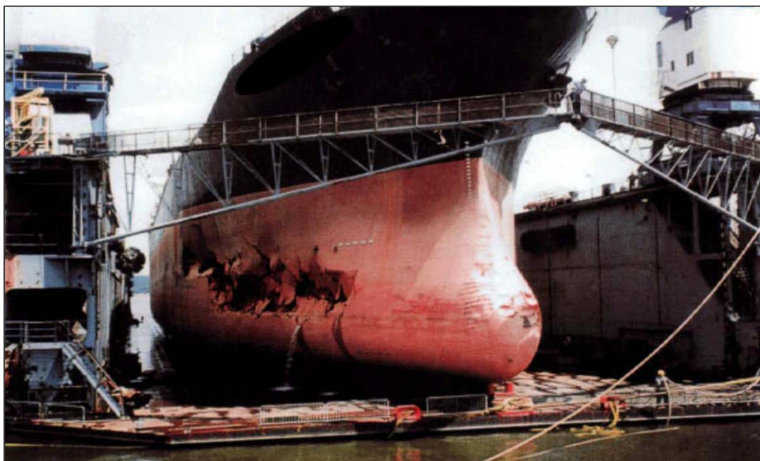
Special coverage is required for damages caused by ice
