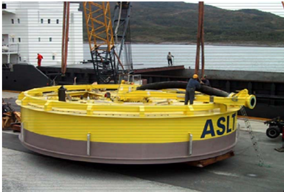
PLEM Loading on board of special carrier for delivery at the site
