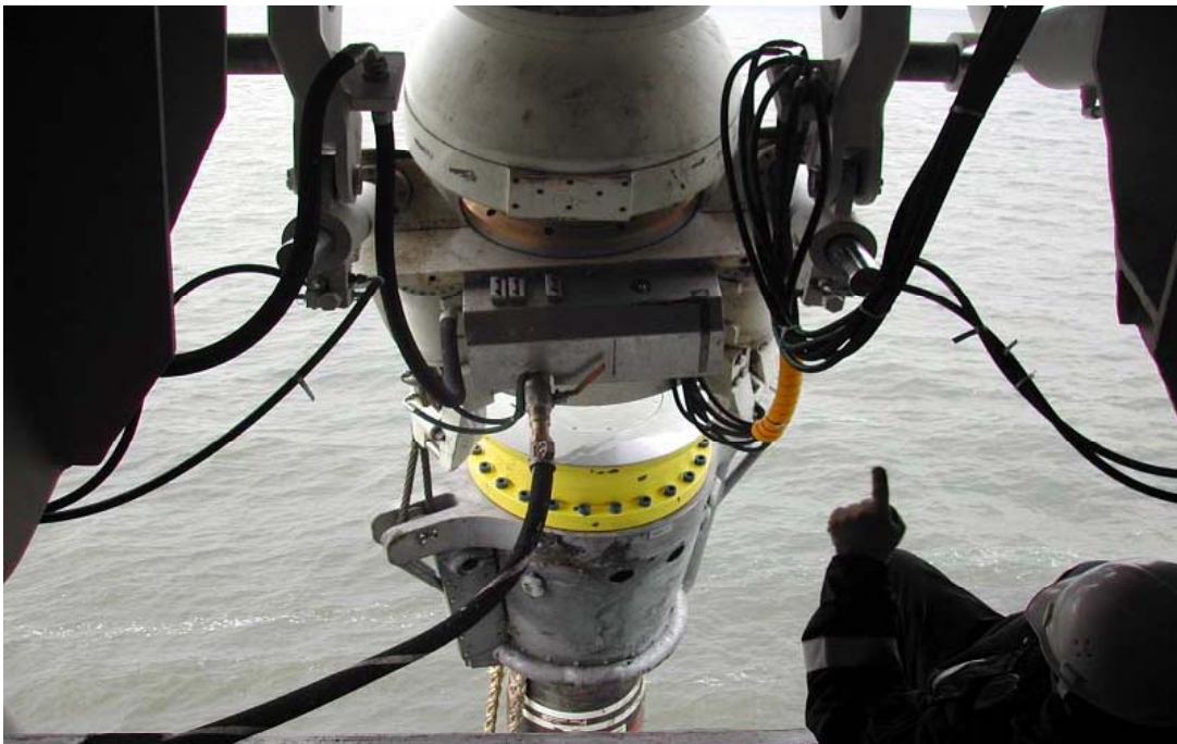
Connecting Mooring Hose to Bow Loading System
