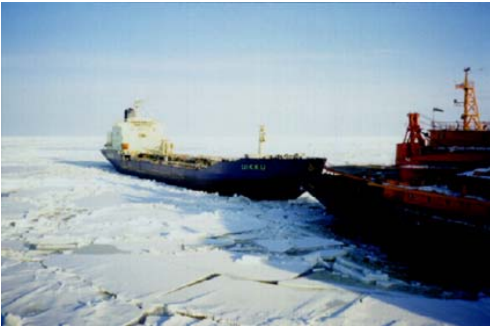
Close towing of tanker Uikku by icebreaker Rossia in the Kara Sea, April 1998
