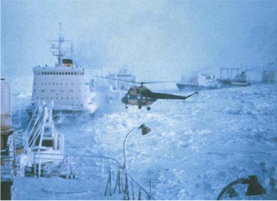
Use of a ship borne helicopter for the search of a lead in drifting ice (tactical ice reconnaissance)
