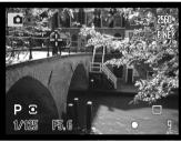
Press the shutter-release button partway down to focus; the FFP turns red briefly to confirm focus.
