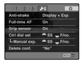
**Exposure** - Anti-shake is only applied during the exposure and is not apparent in the live image. When the shutter-release button is pressed partway down, wait a moment before taking the picture for the Anti-shake system to stabilize the image.
