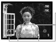
Place the subject within the focus frame. Press and hold the shutter-release button partway down.
