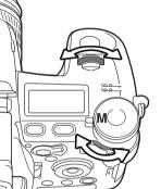
To set the shutter speed, turn the front control dial. To set the aperture, turn the rear control dial. The appropriate display will turn blue as the exposure is changed.
