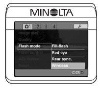
Set the camera to the wireless flash mode in section 1 of the recording menu (p. 80). This will simultaneously set the flash to the wireless mode and set the camera to the flash's wireless channel.
