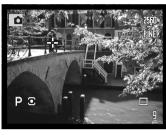
Use the controller's four-way keys (1) to move the Flex Focus Point in the live image.
