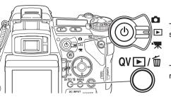
To view images from the playback mode, turn the mode switch to the playback position.
