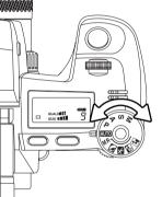
The exposure-mode dial is used to select traditional exposure mode as well as subject programs that optimize camera settings to specific shooting conditions. Camera settings saved in the camera can also be recalled with this dial. Simply turn the dial to the appropriate position.
