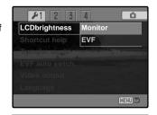
Brightness is controlled in eleven levels. Use the left/right controller keys to adjust the brightness, the monitor will adjust accordingly. Press the central button of the controller to set the level and complete the operation. Press the menu button to close the screen without applying any changes.
