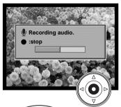
After the instant playback period, a screen will appear indicating the audio recording has started. A status bar will display the amount of recorded time. The recording will stop when the fifteen second recording period has ended or by pressing the center button of the controller.
