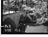
Turn either the front or rear control dial to shift the shutter speed and aperture combination; each combination gives the equivalent exposure. The values are shifted in 0.3Ev or 1/3 stop increments. The front dial changes the shutter speed (Ps) and the rear dial changes the aperture (Pa); the corresponding display turns blue. If the lighting changes, the blue display value remains fixed and the white display changes to compensate for the required exposure.
