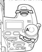
Aperture priority is set with the exposure-mode dial (p. 50). The photographer selects the aperture and the camera sets the appropriate shutter speed to ensure the correct exposure. When A mode is selected, the aperture display on the monitors turns blue.
