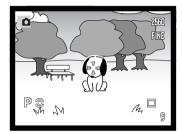
Press the shutter-release button partway down to engage the subject lock; the focus signal will confirm focus. If the subject moves or the camera is panned, the focus area will follow the subject. Focus and exposure will change as the subject moves and lighting conditions change.
