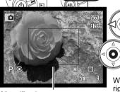
Initially, the 2X magnification area is displayed. This can be moved in the live image with the four-way keys of the controller (1). Pressing the center button of the controller returns the area to the middle of the image. Press the magnification button (2) to enlarge the image.
