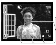
Place the subject within the focus frame. Press and hold the shutter-release button partway down.
