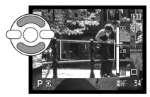
When using the shutter-priority, aperture-priority, or manual exposure modes (p. 36 - 38) with manual focus, press the central button of the controller to switch between using the up/down keys to focus or to adjust the exposure. The active function is indicated in blue.
