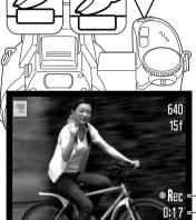
Frame the picture as described in the basic recording operation section (p. 22). Press the shutter-release button partway down to set the the focus and exposure. Press the shutter-release button all the way down and release to start recording.
