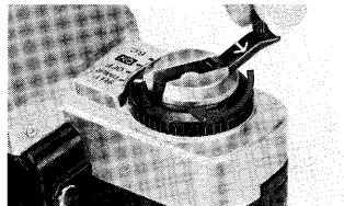
12. Rewind and remove film (p. 41).
