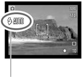
Flash charging - Flash mode indicator is red. Shutter is locked.
