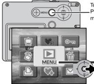
To delete a displayed image, use the main playback menu. Press the menu button to display the main menu on the LCD monitor.
