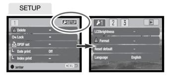
Pressing the controller with the setup tab highlighted opens the setup menu (p. 78).
