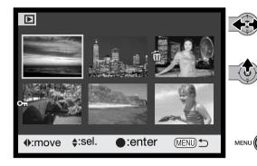
Pushing the controller left and right moves the yellow border to select the image.
