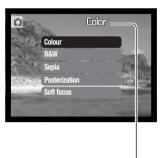
The colour option must be set before an image is captured. When the colour, black and white, sepia, or posterization settings is highlighted, the effect is immediately visible on the monitor. Except for the colour mode, an indicator is displayed on the LCD monitor to indicate the active setting.
