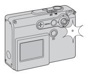
If battery power is very low, the LCD monitor turns off when the flash is charging. The indicator lamp next to the card slot will turn orange and blink quickly when the flash is charging.
