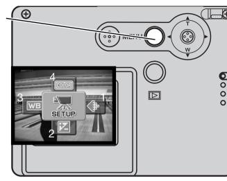
Image size has two settings, 320X240 and 160X120. Image size not only affects the resolution of the movie image, but also changes the maximum length of the movie clip. Recording time is only limited by the capacity of the memory card. A 16 MB memory card can contain approximately 47 seconds of digital video recorded at 320 X 240 or 189 seconds at 160 X 120.
