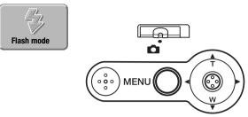
The flash can be used when taking still images. The flash mode is set with the main menu of the recording mode (p. 36). The active flash mode is displayed in the top left corner of the monitor. Flash modes can be assigned to the controller with controller customization (p. 54).
