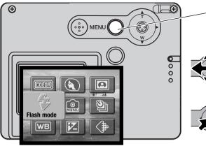
To activate the main menu of the recording mode, press the menu button.
