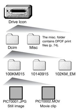
Files and folders on the memory card can be deleted using the computer. Never format the memory card from the computer; always use the camera to format the card. Only files recorded by the camera should be stored on the memory card. Image file names begin with "PICT" followed by a four-digit file number and a jpg or mov extension. The jpg extension indicates a still image, and the mov extension, a movie clip.
