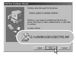
The last window will confirm the driver has been installed. Click "Finish" to close the add new hardware wizard. Restart the computer.
