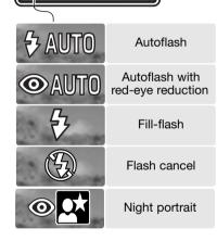
Autoflash - the flash fires automatically in low-light and backlit conditions.
