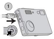
Turn the camera on. Open the PictBridge menu (p. 100). Highlight "Start" in the DPOF-print option in section 3 of the menu. Press the controller to continue.
