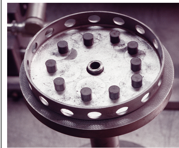
Uranium-plutonium mixed oxide (MOX) fuel pellets for nuclear reactors, made from excess weapons plutonium. The United States should offer to finance the costs of disposition of Russia's excess plutonium, as the $1-$3 billion cost of the project is small by comparison to the security risk posed by this dangerous stockpile. Source: Los Alamos
