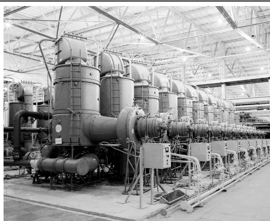
Diffusion machinery for uranium enrichment in the closed city of Novoural'sk (formerly Sverdlovsk-44). The United States should offer to buy substantial additional quantities of Russian HEU, with a part of the proceeds to go to fund nuclear security activities such as ensuring that nuclear guards are paid—with reciprocal monitoring at U.S. and Russian facilities to confirm that no new HEU is being produced. Source: DOE
