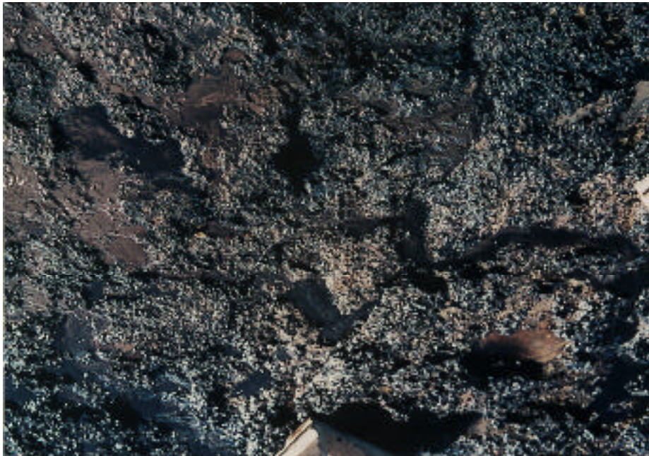
Figure 20D. Close-up of the Corexit 9580-treated beachrock surface during flushing operations. Note that some of the oil has dispersed, forming brown, muddy wash water in addition to black oil.
