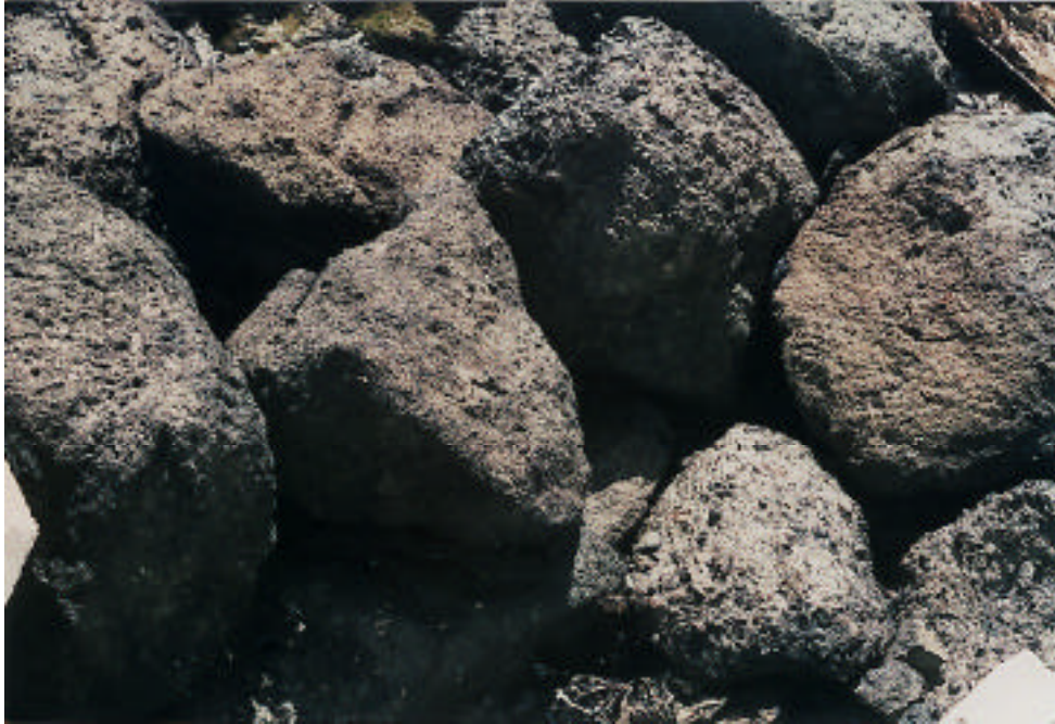
Figure 21C. Plot for the Corexit 9580 cleaner on rip rap; washing was conducted up to 1,200 psi and 175°F water.
