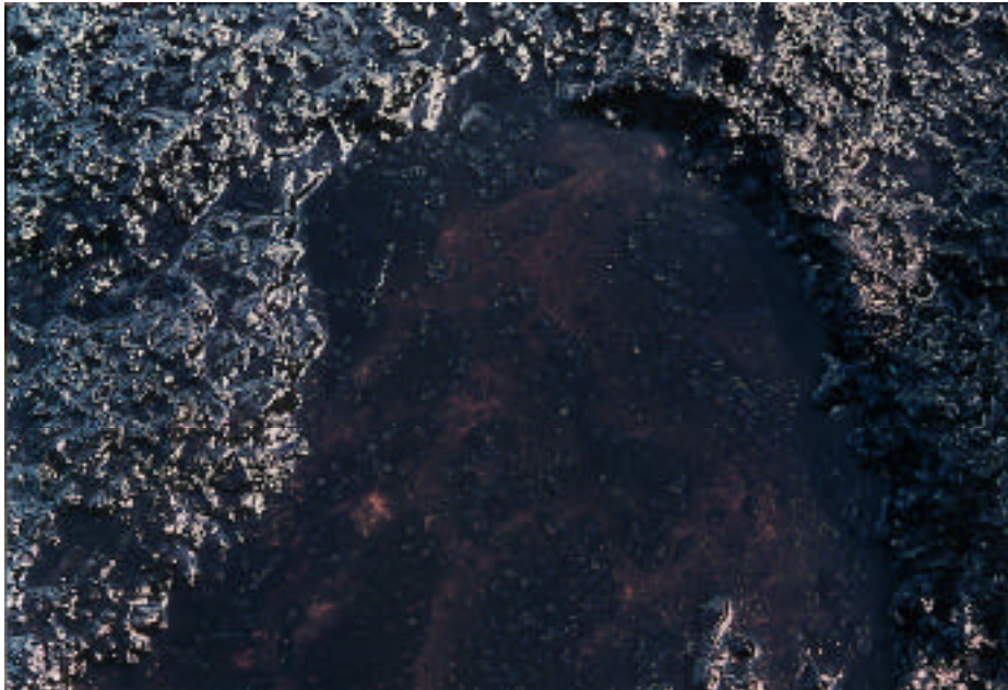
Figure 20F. Close-up of the PES-51-treated beachrock surface during flushing operations. None of the oil was dispersed, even at 1,000-psi water pressures. Treated and released oil was liquid and black, with small bubbles attached to floating slicks.
