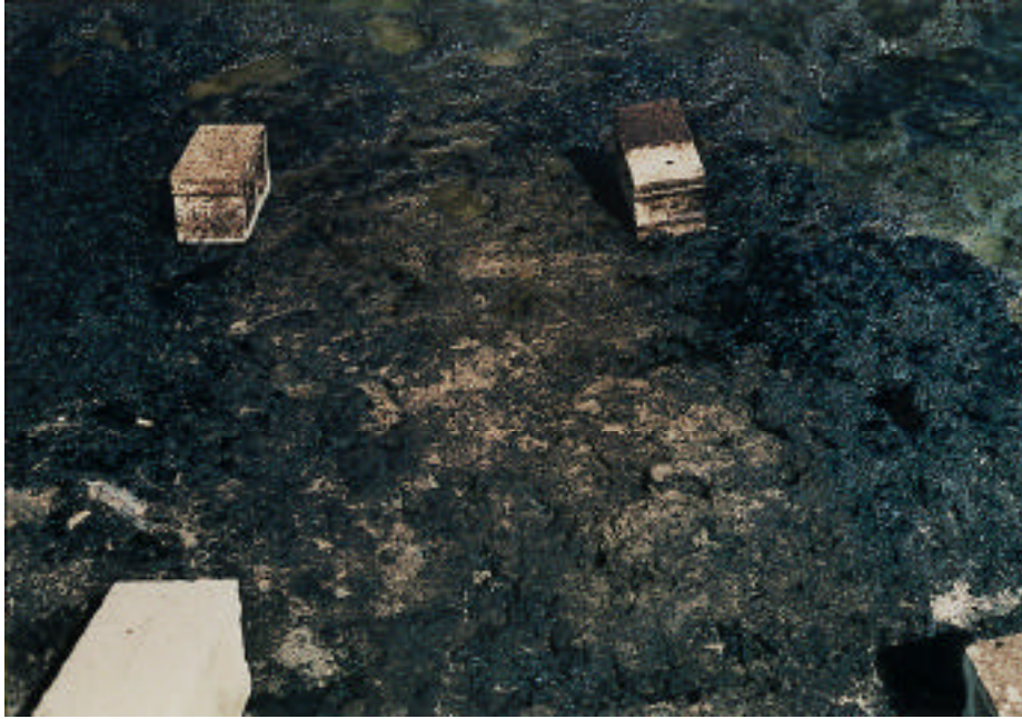
Figure 20C. Plot for the Corexit 9580 cleaner, which was flushed with high-pressure, hot water: the left side of the plot at 500 psi and 140°F; the right side at 1,000 psi and 175°F. The right side was significantly cleaner without any chipping of rock. The worker tended to sweep the entire area with the spray because oil was continually released during washing.
