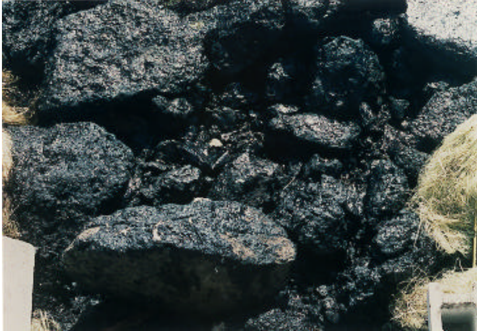
Figure 21A. The rip rap washing test reference plot. No pressure washing of any kind was conducted. All the plots had been cleaned to the extent possible by manual wiping.
