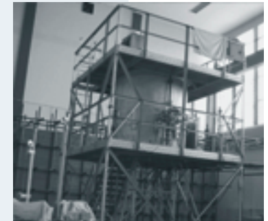
This Vinca critical assembly research apparatus once operated on weapons-grade HEU fuel. As a result of Project Vinca, it has been converted to proliferation-resistant low enriched uranium fuel.
