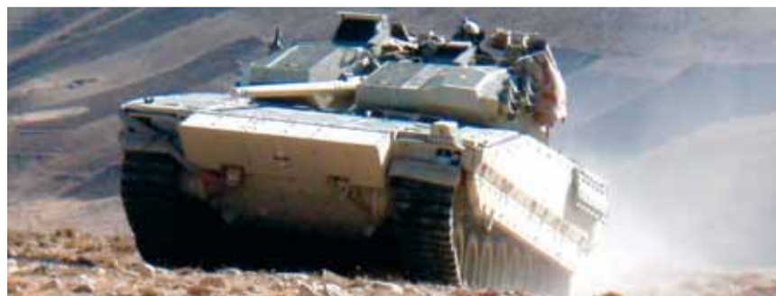
Above: the rubber tracks cut noise, improve stealth, reduce crew fatigue and increase mobility
