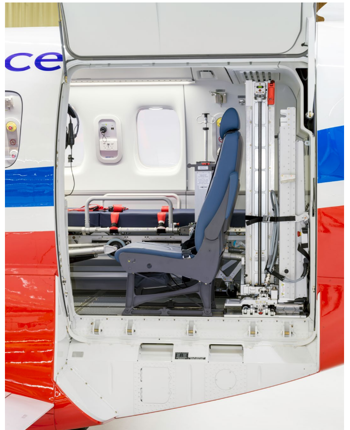
Electric stretcher loading device retracted with additional quick-change seat
