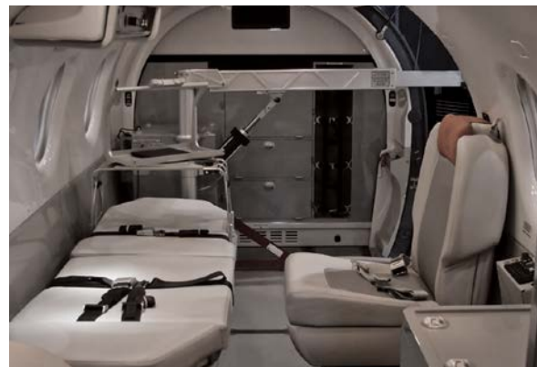
The medevac configuration provides room for two patients, attendants, and equipment.
