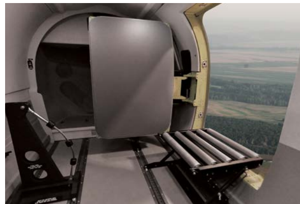
An optional integrated utility/jump door increases the number of roles the Spectre™ can accomplish while retaining the standard cargo door functionality.
