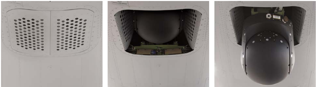
The retractable EO/IR sensor deploys quickly in flight, and retains a covert profile on the ground.
