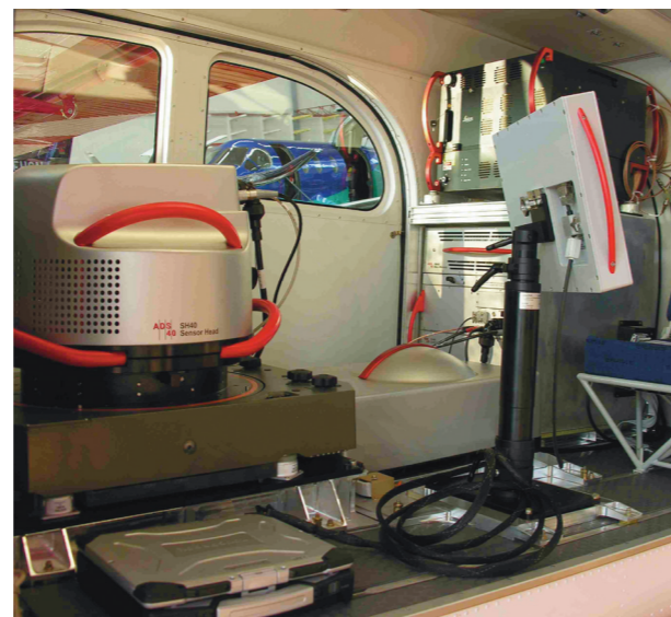
Installation of a static aerial photography system
