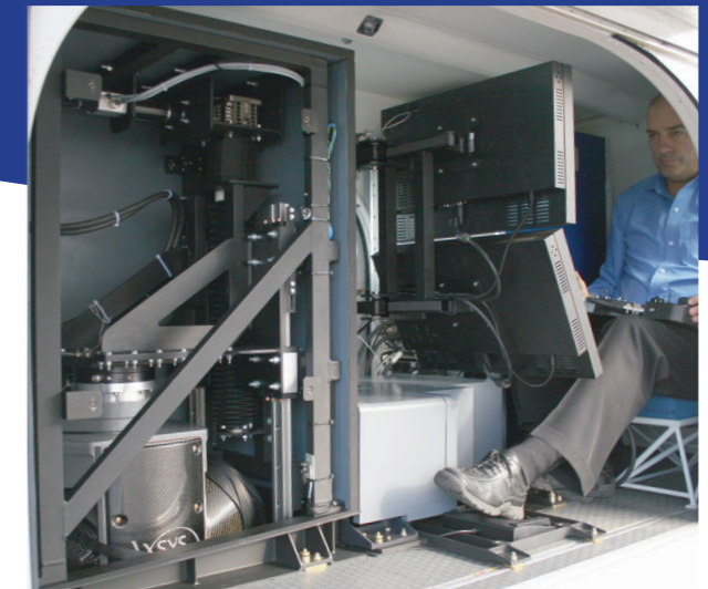
Dynamic camera system on retractable platform which can take different sensor heads up to 80 kg
